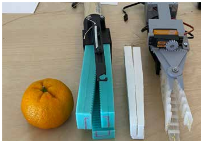
Figure 7: Left: A soft-fingered fruit gripper with a “crochet hook” style cutter and silicone-covered fingers. Center: the silicone finger coverings. Right: Bare flexible fingers and a scissors-like stem cutter. Mandarin fruit included on far-left side for scale.
