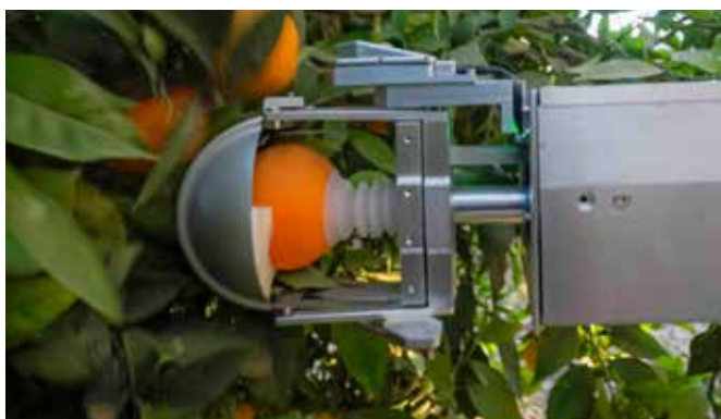
Robotic end-effector in action; vacuum sniffer is securing an orange for picking via cutting its stem by blades.
