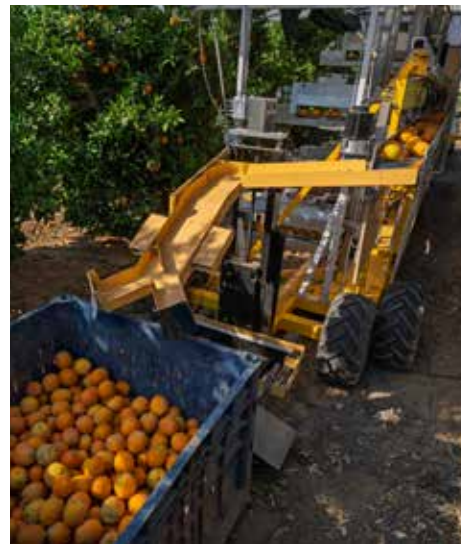
Harvested fruit gently being transferred into bins via an integrated conveyor system.
